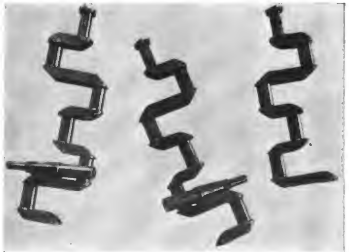
FIG. 4.—Three from a batch of more than a score, all of which broke in the same place in little more than a month.
